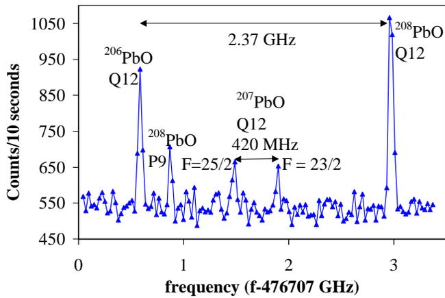
FIG. 1: A scan over the Q12 transition of the  $X(0)(v'' = 2) \rightarrow a(1)(v' = 3)$  transition. The  $^{208}\text{PbO}$  and  $^{206}\text{PbO}$  lines are prominent, with the smaller  $F = 23/2$  (higher frequency) and  $F = 21/2$  lines of  $^{207}\text{PbO}$  split by the hfs. The  $^{208}\text{PbO}$  P9 transition is also apparent.
