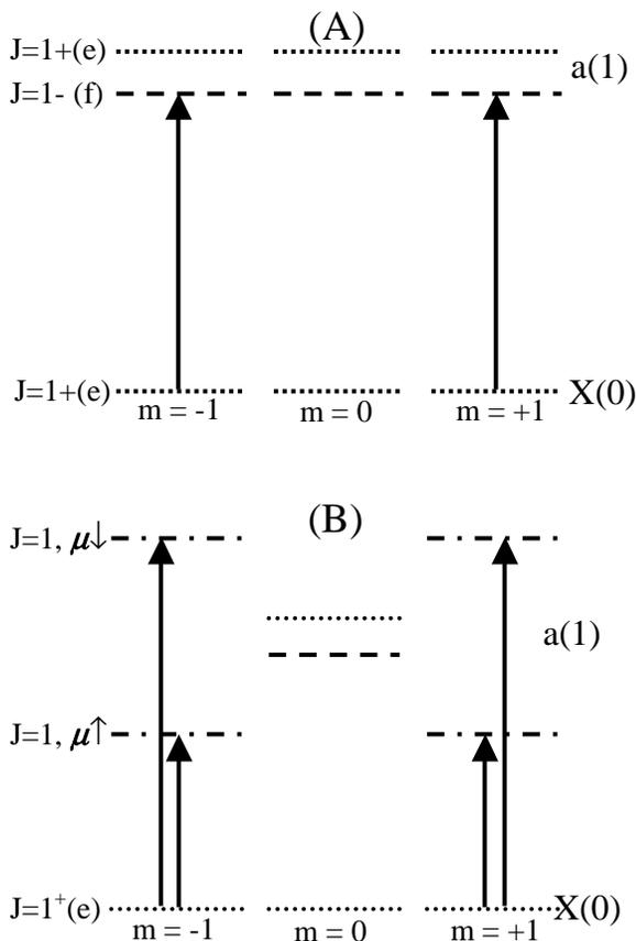
FIG. 3: Schematic description of the Stark effect on the Q1 line, with z-polarized light. (A) Q1 line with no electric field. (B) Q1 line with  $\mathbf{E} = E\hat{z}$ . Sublevels with equal values of  $|m|$  remain degenerate.
