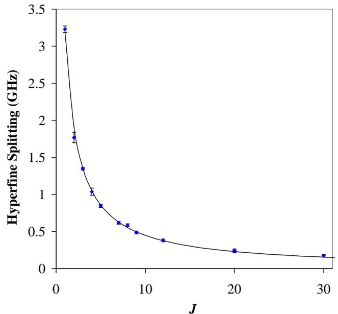
FIG. 2: The hfs of the  $a(1)(v' = 3)$  state of  $^{207}\text{PbO}$  as a function of the rotational number  $J$ . The solid line is the prediction using Eqs. 1-3 and the best-fit value  $A_{\parallel} = -4.11(3)$  GHz.
