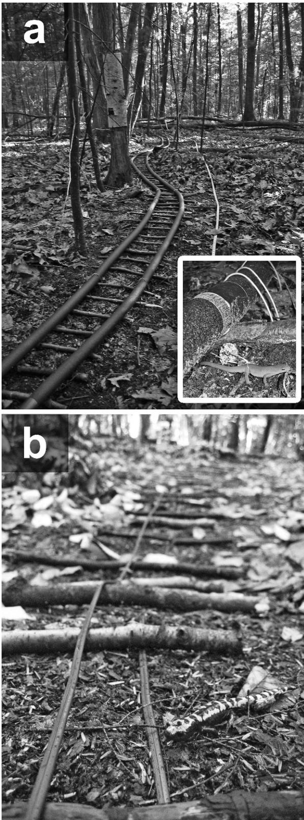
**Figure 2.** Examples of passive integrated transponder (PIT) antennae in the field. A tagged juvenile red-spotted newt crosses under the full duplex (FD) antenna at the S. O. Conte Anadromous Fish Research Center in Turners Falls, Massachusetts, USA (a). A tagged adult marbled salamander approaches a half duplex (HD) antenna in the Holyoke Range in Massachusetts (b).
