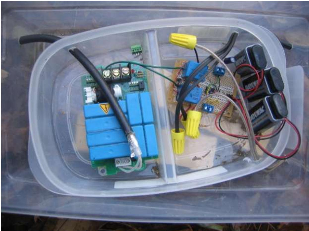
Figure 2. HD Switching setup. Left side are tuning capacitors, and lead to readers, right side is switching circuit and leads to antennae.
