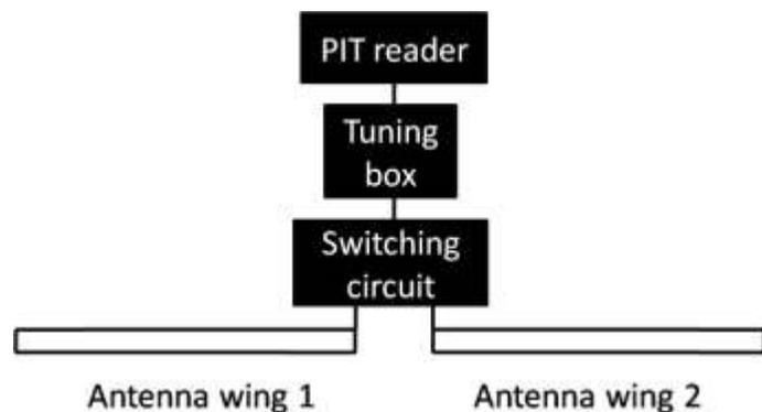
Figure 1. Basic antenna setup employed in our study.
